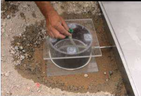
Installation of the water collecting unit
